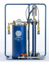
HOW IT Establish safe work area, Begin test. Start recording continuous mass readings for wet space that measures any change in mass Inject nitrogen for pressure or draw vacuum into ullage space to measure any change Continue simultaneous testing of wet and ullage space for relevant period. Technician receives real time results, diagnoses any leaks/issues Data uploaded to cloud and analysed by qualified Digital report sent to customer
